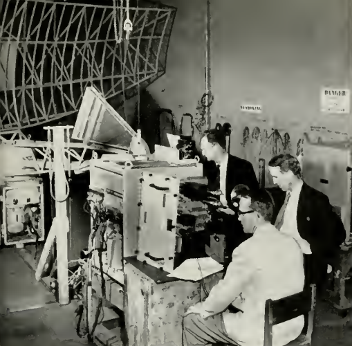
Above, a government inspector looks on as radar set control and pedestal are tested at RCA Victor Montreal plant. At right, new RCA antenna provides communications link in British Columbia.
